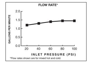
1.5 gpm/5.7 L/min. FLOW RATE
